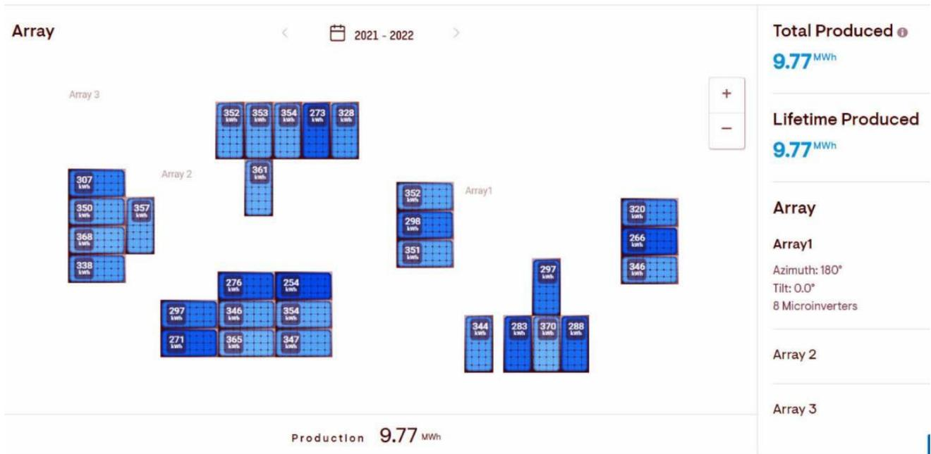
Since measurements started on July 12, 2021 (11 months ago), the system has generated 9.77 MWh, with each panel ranging from 254 to 370 kWh per year.
